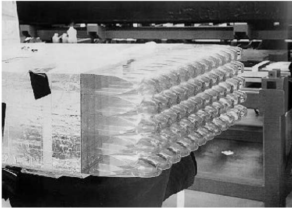
Fig. 3. Light guides at one end of a barrel module before photo-tube installation.
