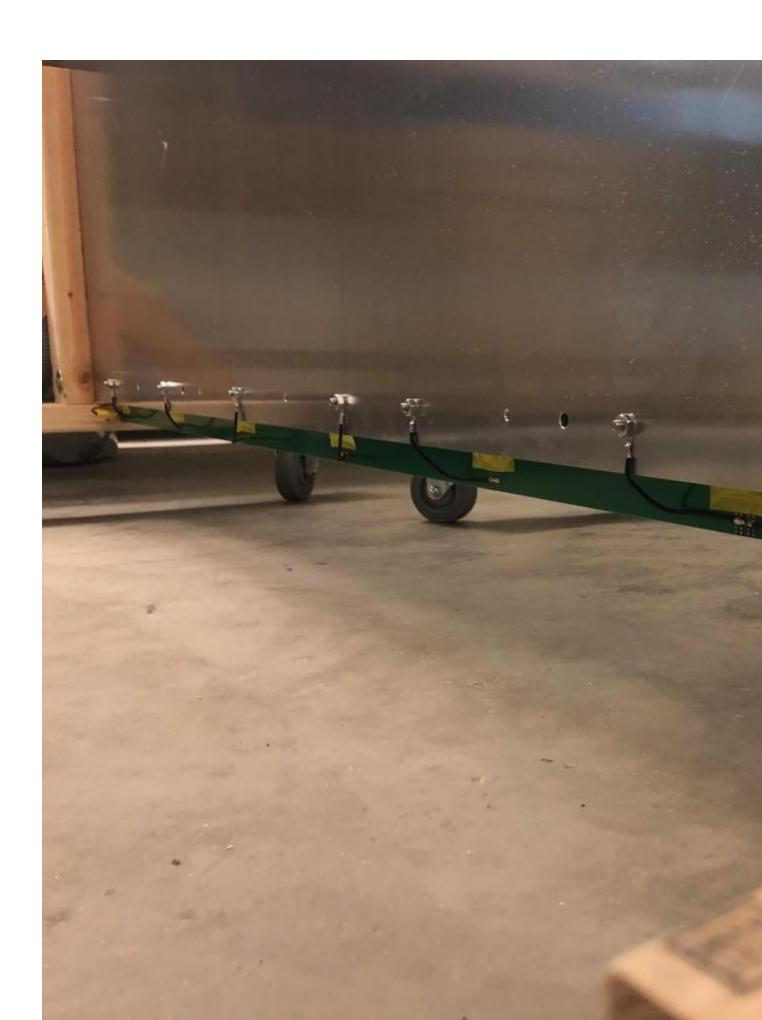
I know at the last meeting there was discussion that the two sides of the chamber would be completely flat, with nothing extending beyond the surface of the aluminum plates. This is going to be difficult to do, given the need for fastening the shielding box to the detector, and providing a good grounding connection to the electronics.
