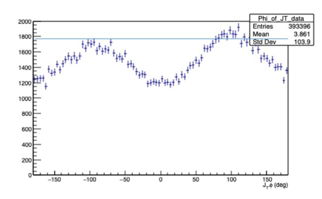
Offset from collimator is probably along 135 deg (or maybe 225?), not 45 deg. The ebeam collimator offset is likely larger than 1mm!
