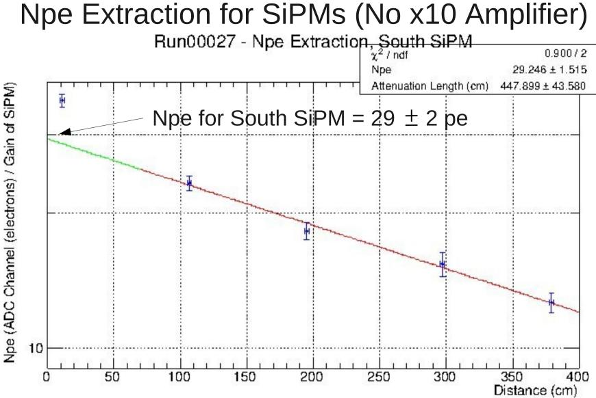
Assuming a single-exponential behaviour, the number of pixels fired in the SiPM (Npe for ease of explanation) for a MIP which occurs very near the edge of the module (at distance ~ 0 cm) is the y-intercept in the plot of Npe vs. Distance
