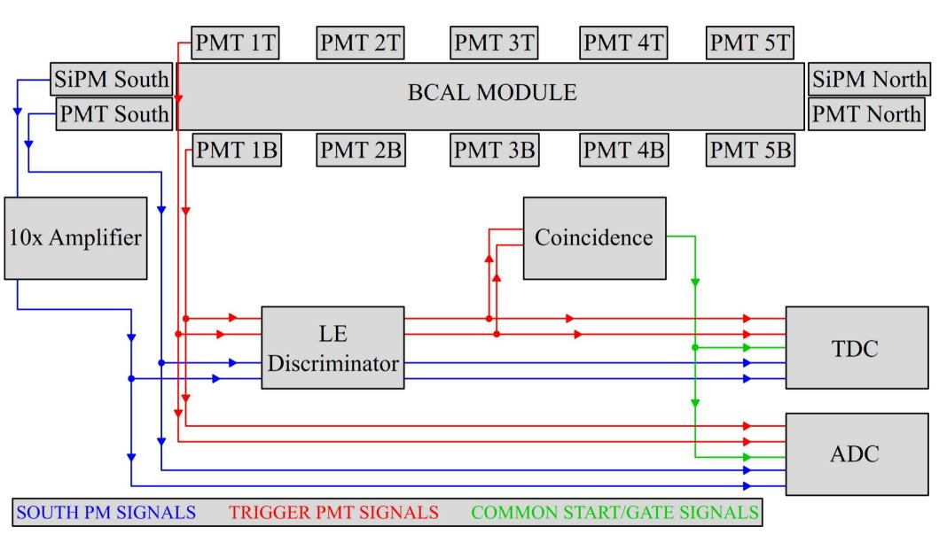
Shown for one trigger pair and the south photomultipliers. The other four trigger pairs and the north photomultipliers have identical setups
