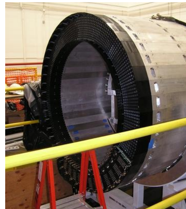
Barrel calorimeter (BCAL) 11^\circ < \theta < 125^\circ
