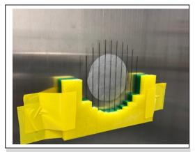
Carbon fiber tubes used to deaden drift chamber wires in beam region. The size and shape of the dead region as well as other design parameters were optimized using A.I.
