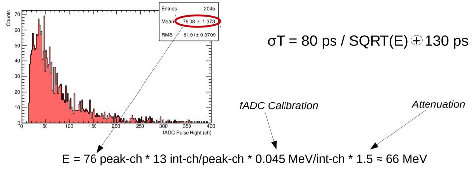
Mean-Time Resolution:  $\sigma T = 80 \text{ ps} / \text{SQRT}(0.066) \oplus 130 \text{ ps} = 337 \text{ ps}$
