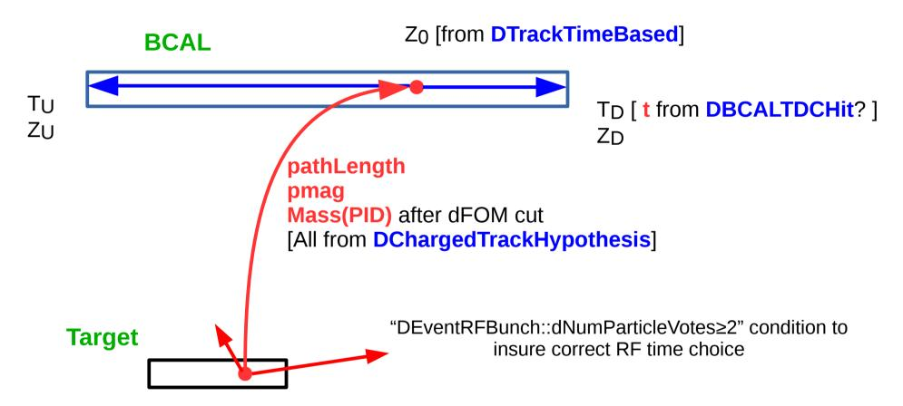
T: chosen RF time, propagated to the z-vertex of the track in the target [T from DVertex or to from DChargedTrackHypothesis?]
