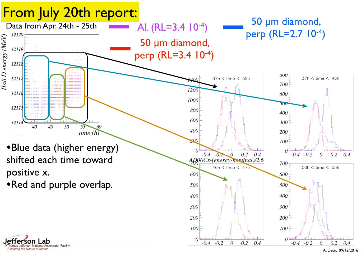
Variation of beam position at tagger dump with radiator thickness:
