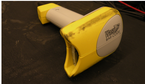
Figure 8: The barcode scanner used to read in the PMT IDs efficiently.
