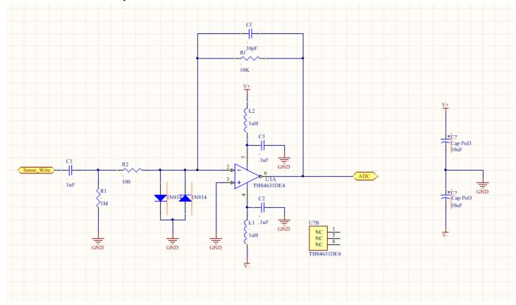
Major changes include the addition of ferrite beads of the Op Amp power supply traces to minimize interference between the channels. Also, diode protection was added to the input of the amplifier.
