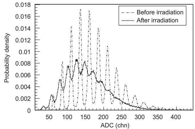
**Fig. 6.** ADC spectra for low amplitude signals from green sensitive Photonique SiPM before and after irradiation with  $3.1 \times 10^9$  electrons/mm<sup>2</sup>.
