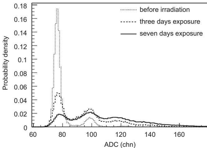
**Fig. 8.** Noise spectra of a green sensitive Photonique SSPM-0701BG-TO18 device that was exposed to mixed background irradiation close to the beam-line during one week of normal beam operation. Substantial damage was observed after 3, respectively, 7 days of exposure.
