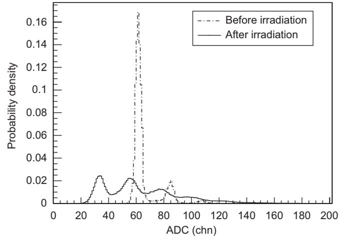
**Fig. 5.** Integration of dark pulses in a randomly generated window for a bias voltage of 17.9V before and after irradiation with  $3.1 \times 10^9$  electrons/mm<sup>2</sup>. The reduction of the pedestal amplitude relative to the one or more pixel peaks and its shift in position are a result of the increase in dark count rate.
