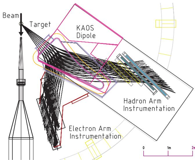
**Fig. 1.** Overview of the KAOS spectrometer operated by the A1 collaboration at the Mainz microtron MAMI: electrons and hadrons are detected under small scattering angles in coincidence. Charged particle trajectories through the spectrometer are shown by full lines. The electron arm tracking detector will be located close to the electron beam. High radiation levels are expected at such an exposed position.
