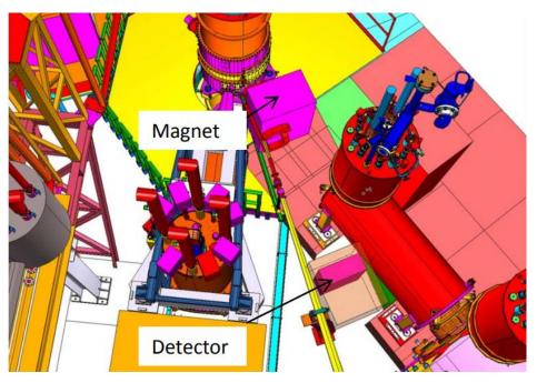
Design based on 2x2x20 cm PWO crystals optically coupled to PMTs
