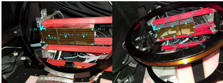
Figure: Units listed are in gauss and correspond to the field strength achieved with our 3A setting. Orientation 1, "field facing PMT" (left). Orientation 2, "field facing down" (right).
