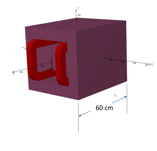
**NOTE**: Physics requests void between coils to be filled with WCu for radiation shielding.
