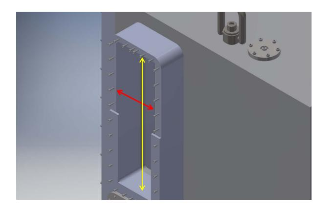
**Clearance on red dimension:** 5.827 in. (opening) - 5.591 in. (flange) = .236 in. or ~6 mm
