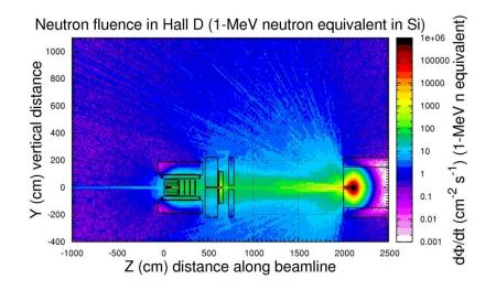
• Estimated background from liquid hydrogen, helium, and deuterium targets using Fluka and Geant simulations provided by the JLab Radiation Control group
