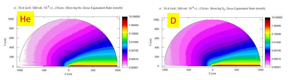
Estimated neutron dose equivalent rate in Hall D(ceiling) produced in the deuterium target is expected to be 3 – 4 times larger than that for helium (conservative assumption)
