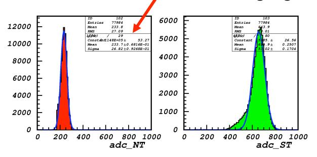
Mean\_ADC (North) ≡ ADC1 = (234-17) = 217 channels Mean\_ADC (South) = ADC1 \* R\_pmt \* R\_far\_near = (656-17) = 639 ch
