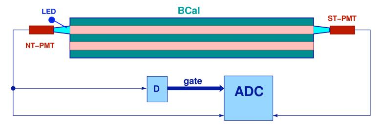
PMTs: non-calibrated Burle 8575 (used previously in the Bcal tests with cosmics)
