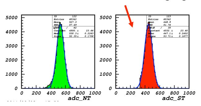
Mean\_ADC (North) = ADC1 \* R\_led \* R\_far\_near = (530-17) = 513 ch Mean\_ADC (South) = ADC1 \* R\_pmt \* R\_led = (447 - 17) = 430 ch
