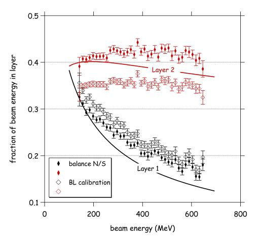
Figure 3: Fractional energy deposition using equation 2 compared with fractional energy deposition for the first two BCAL layers using calibration from N/S balancing (filled diamonds) and using calibration from the minimization technique (open diamonds).
