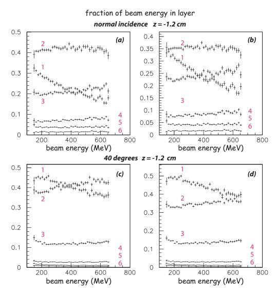
Figure 4: Fractional energy deposition in the six layers as a function of beam energy for normal incidence at z = -1.2 cm using calibration from (a) North/South balancing and from (b) minimization and at 40° at z = -1.2 cm using calibration from (c) North/South balancing and from (d) minimization.
