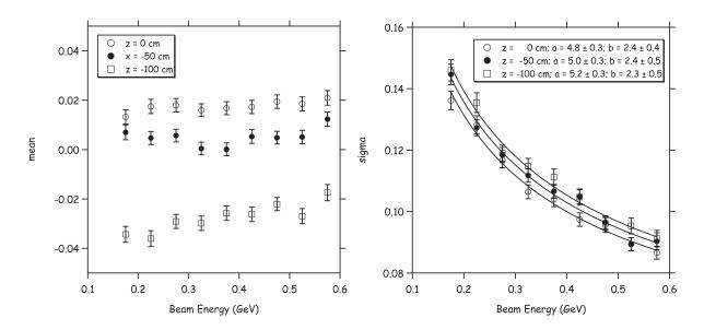
Figure 6: Results of Gaussian fits to the distribution in the quantity defined by equation 1 for bins of beam energy. The resulting mean (left panel) and sigma (right panel) as a function of beam energy are shown. For the sigma, the curves are the results of fits to equation 4.
