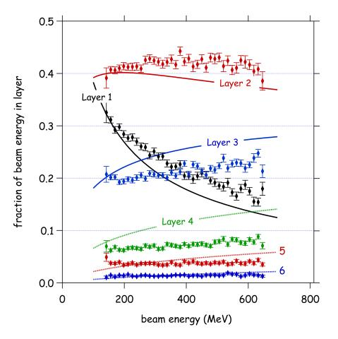
Figure 2: Fractional energy deposition per BCAL layer as a function of photon beam energy for Run 2334 after N/S gain balancing. The curves are the expected results using equation 2. This can then be used to adjust/check layer to layer calibrations.
