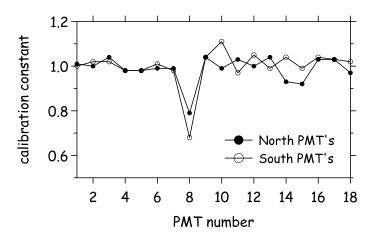
Figure 1: Calibration constants for individual BCAL PMT's determined by minimizing the width of the distribution in the quantity defined in equation 1.
