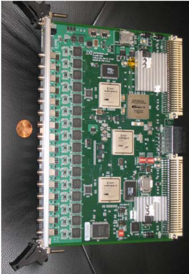
16 channel 250 Mps Flash ADC
