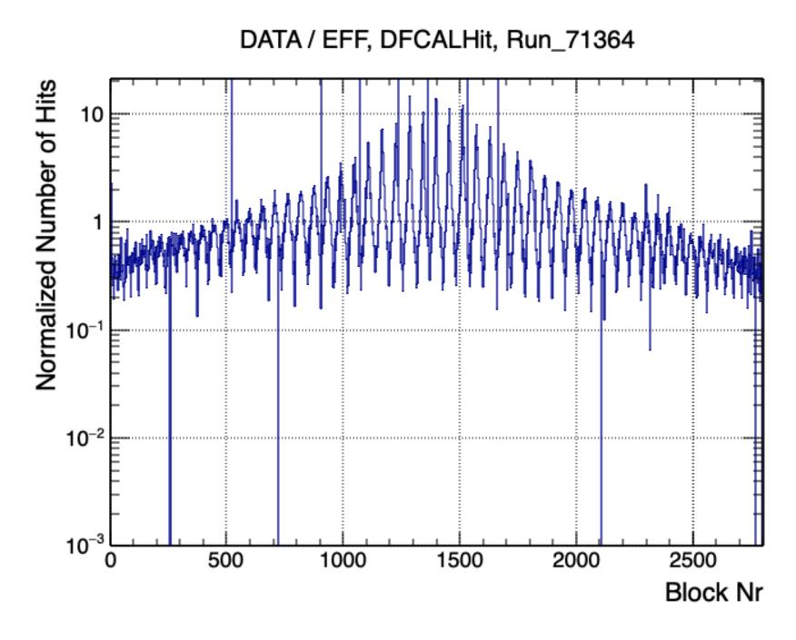
LED block efficiencies, average per run used in simulations
