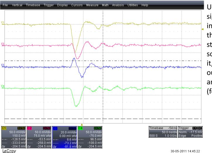
Using the MPPC, signals were injected into amplifiers and the output was been studied in order to set some parameters of it, this are matching output impedance and amplification (feedback resistor)
