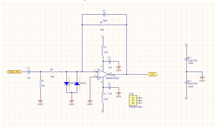
Major changes include the addition of ferrite beads to the Op Amp power supply traces to minimize interference between the channels. Also, diode protection was added to the input of the amplifier.
