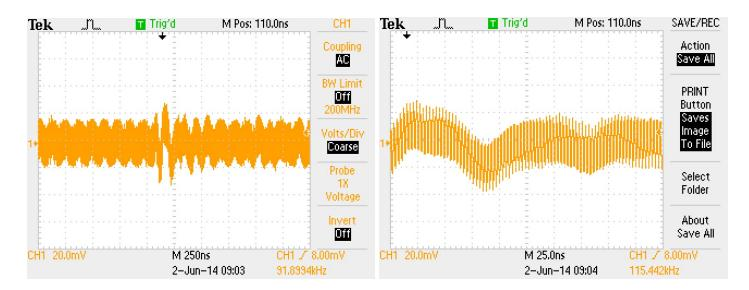
Difficult to visualize the feedback frequencies using just the waveform, use fourier analysis to visualize these frequencies:
