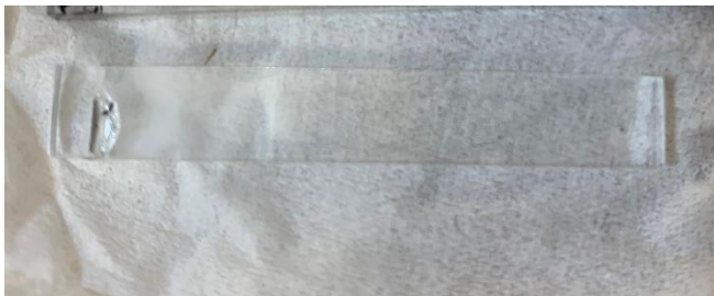
Figure 6. Towards the left part of the scintillator is a chip missing where it would have rested against the edge of the slot of the light-guide.
