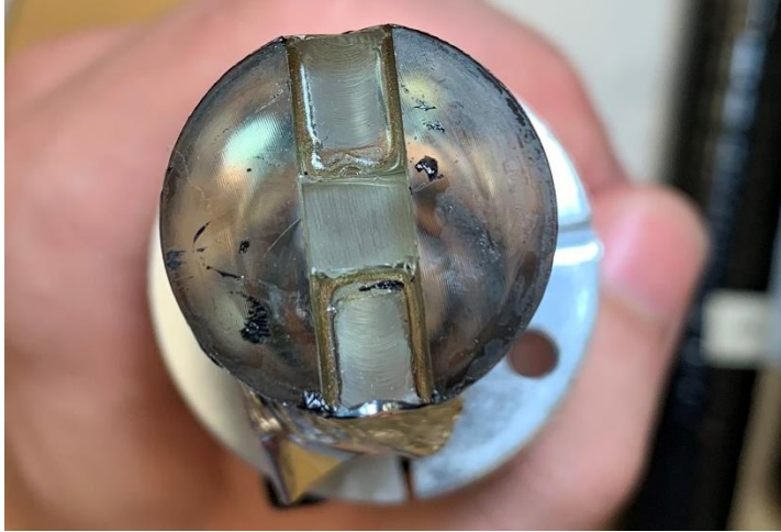
Figure 7. View of counter 98's light-guide. The indentation in the epoxy is where the scintillator once rested. Also note the black-electrical tape adhesive found on the light-guide.
