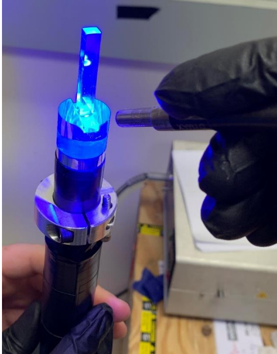
Figure 14. Picture showing the UV pen being used on the epoxy that mounts the scintillator to the light-guide securely.
