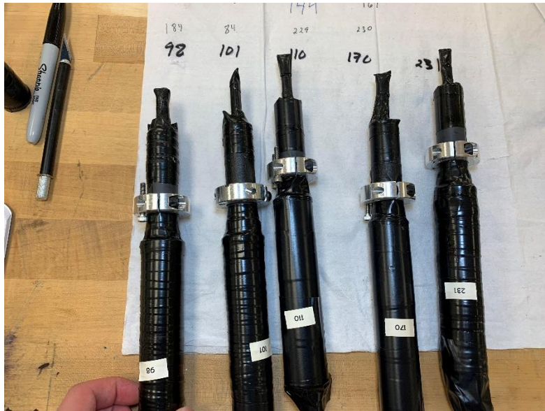
Figure 1. Initial state of the scintillator counters before any work was done to them.
