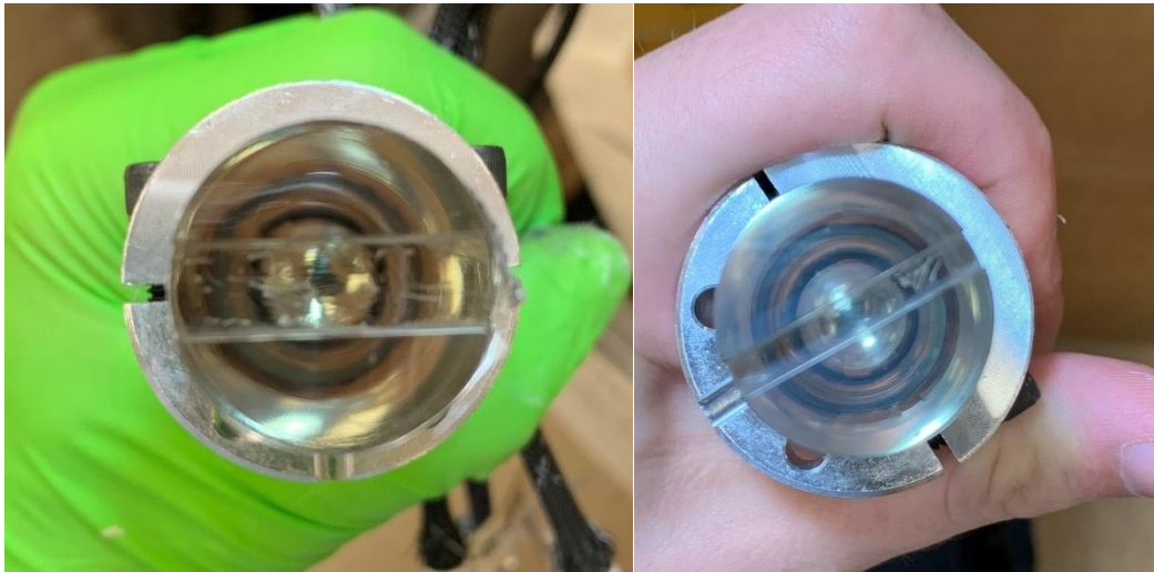
Figure 12. Comparison between scratches left by exacto knife, left picture, and poking tool for removing epoxy from the light-guides, right picture. Both have been polished.
