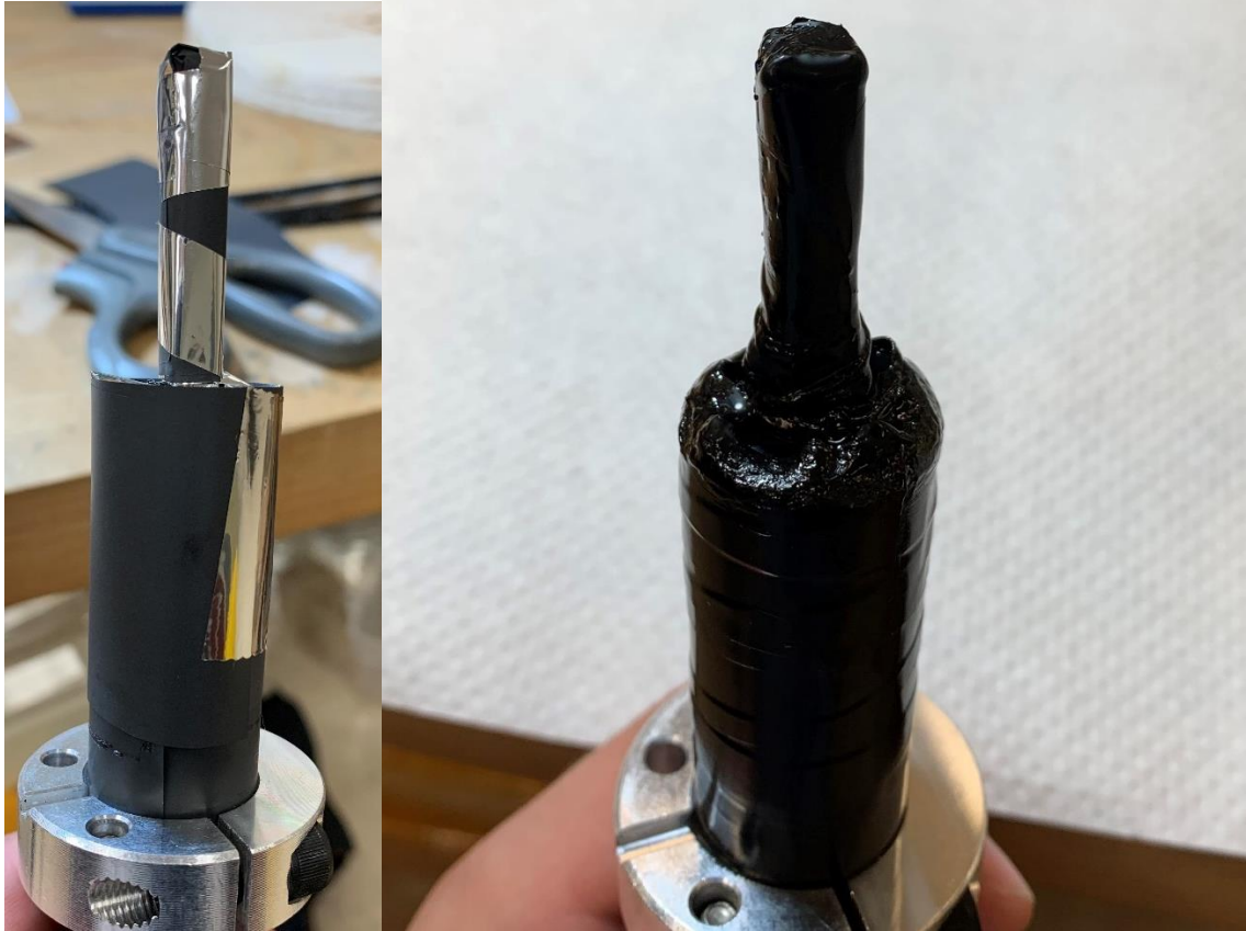
Figure 16. The picture to the left shows the tedlar around the scintillator and cylindrical portion of the light-guide. A mylar tape was used on the tedlar. The right picture shows the black electrical tape wrap starting at the joint and extending up to the base of the scintillator. The scintillator and top of portion of the light-guide were then covered in liquid black electrical tape.
