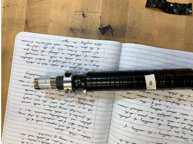
Figure 2. Counter 98 with its electrical tape above the collar removed as well as most of its tedlar.
