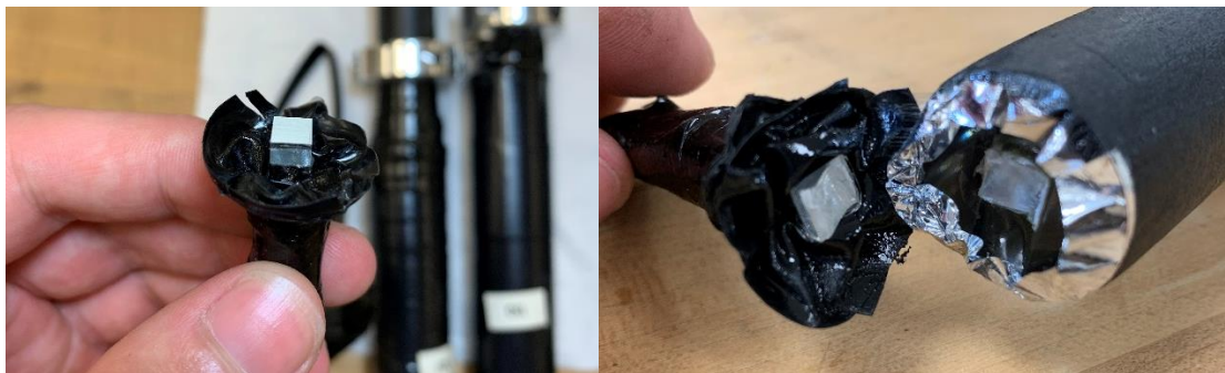
Figure 3. The picture on the write shows how the scintillator, from counter 98, just came right out of most of the counters with just a small amount of force. Also note, there is a white film on the scintillator in the left picture. The picture on the right shows a scintillator that was found to have been split into two pieces.
