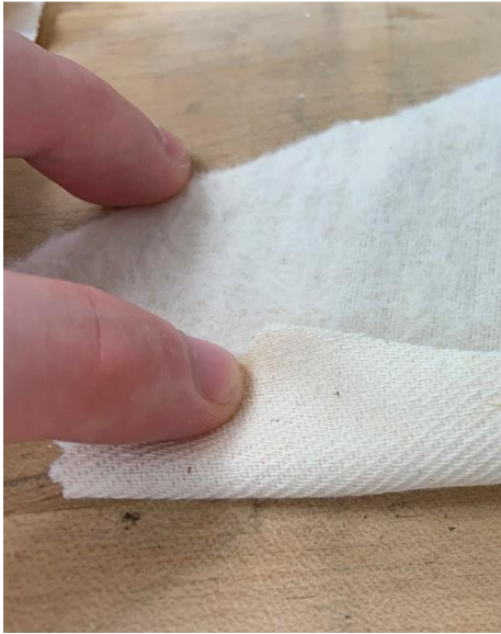
Figure 9. This is a picture of the cloth used to polish the light-guides and scintillators. The soft side was used for rubbing against the surfaces with the polish.
