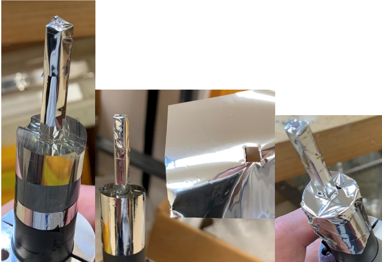
Figure 15. This figure shows pictures in order of the processes detailed above. First mylar is wrapped around the scintillator, then cylindrical part of the light-guide, followed by the top part of the light guide. Everything is taped using a mylar tape.
