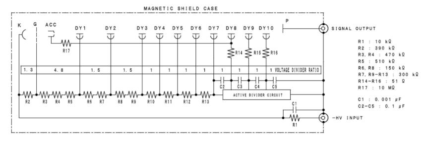
VOLTAGE DIVIDER CURRENT = -390 μA at -2000 V (MAX) INPUT
