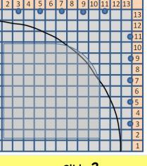
Dots represents the limit of the area occupied with FCAL PMTs
