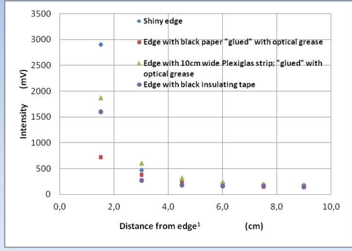
Short PMT@1340V (30mm  $\times$  30mm window)  $^1\text{Distance of the PMT window central line from the Plexiglas edge Blue LED, Intensity in mV$
