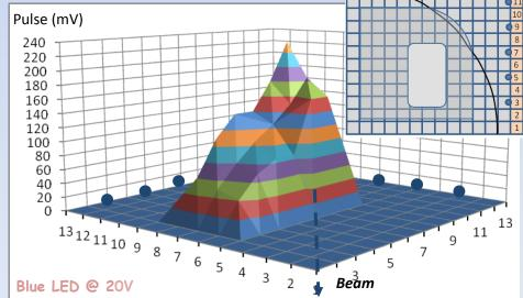
Measurements taken in the middle of  $10 \mathrm{cm} \times 10 \mathrm{cm}$  grid at position expected to be occupied by FCAL PMTs.
