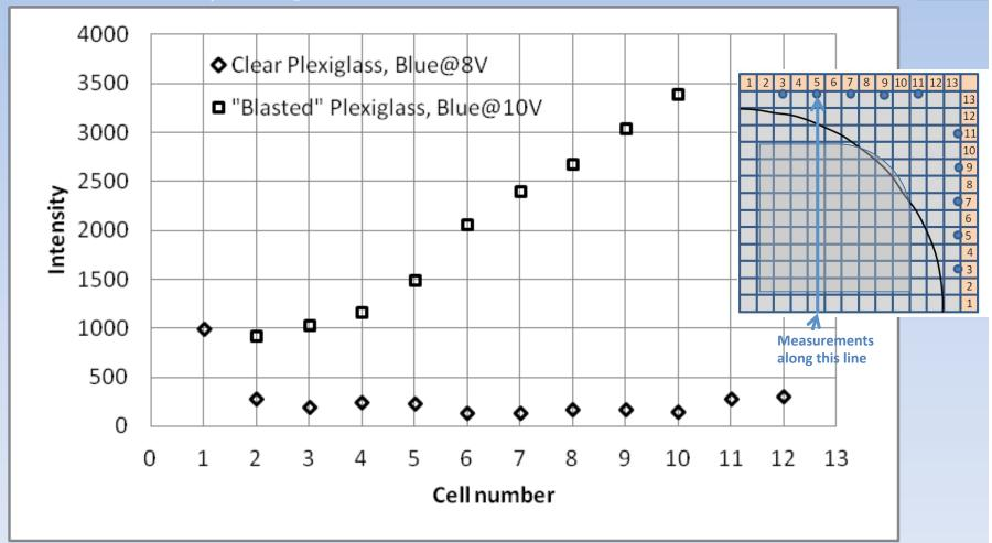
Short PMT@1340V Blue LED Intensity in mV
