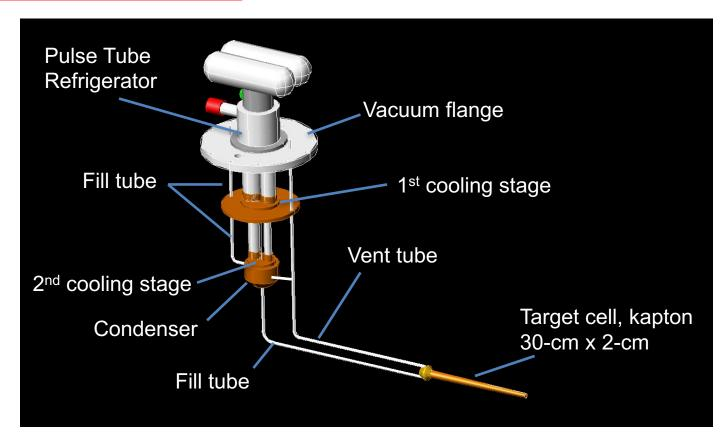
In the case of LHe, only the target cell is filled with liquid. Subcooling is not possible, and the liquid is on the SVP curve. Some boiling is present.
